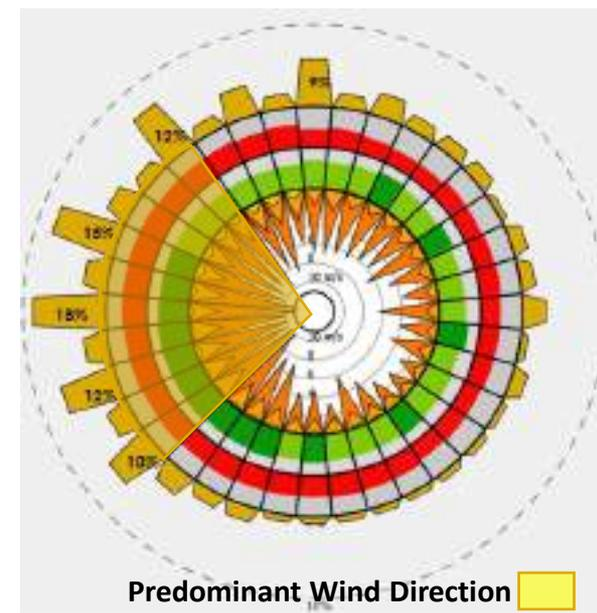
CFD INPUT CONDITION (Max. Avg. Wind Speed: 4.16m/s; Wind Direction: South West – North West (SW-NW))
