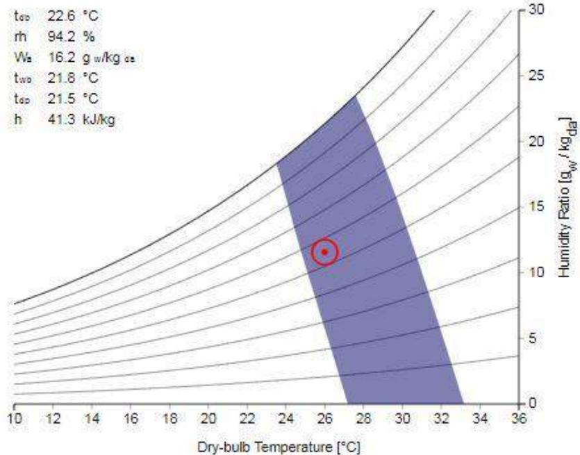
**Conclusion** - The Thermal Comfort Analysis shows that to maintain comfortable range inside the building, the temperature should be maintained as per the thermal band. The thermal comfort can be achieved in all the spaces keeping the thermostat at 26 deg. C.
